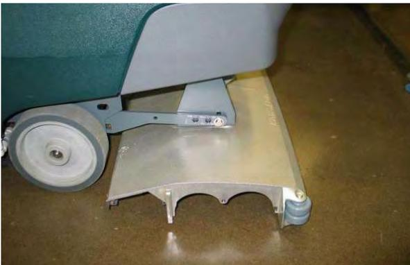
5. Remove front shroud mounting hardware (2).
