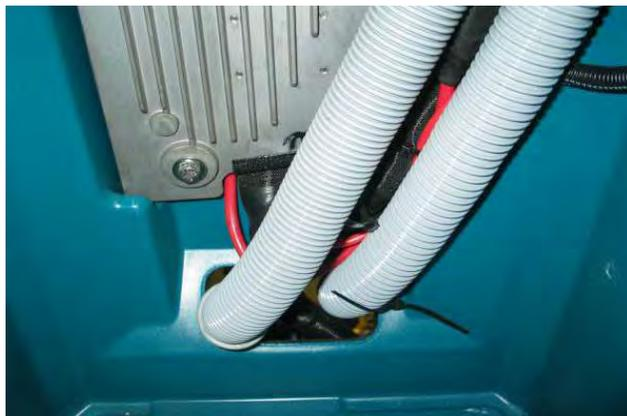
5. Remove the heat sink mounting bolts (2).
