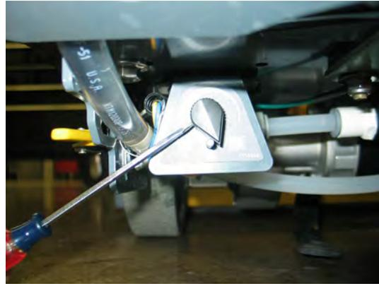
9. Reconnect PTC (Push-To-Connect) fitting to water solenoid valve, cut zip tie securing bail handle, and reconnect transaxle motor connection. Adjustment is complete.
