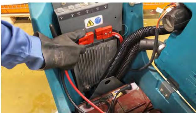
3. Remove batteries and set aside.
