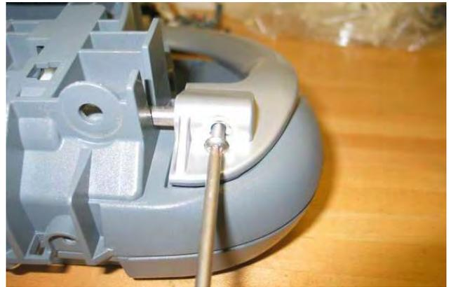
12. Remove screws (4) from front of operator's console.
