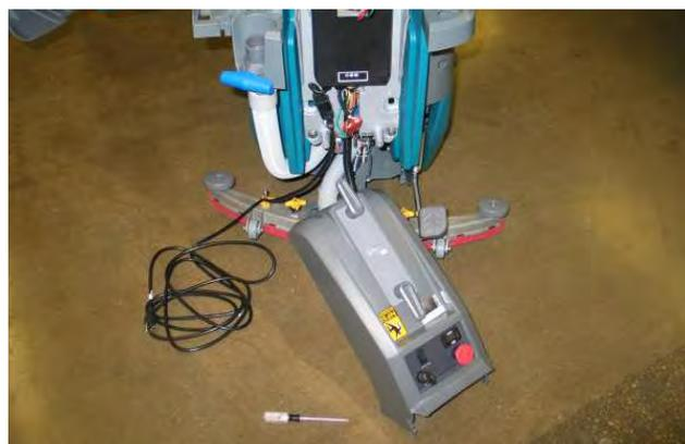
4. Disconnect charger electrical connections.
