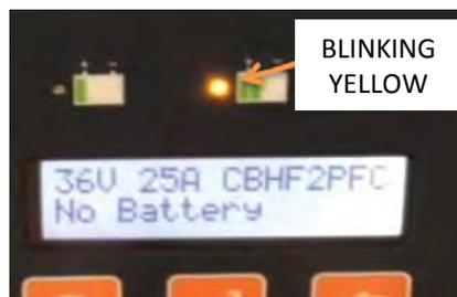
2. Press and hold the two outside arrows for 12 seconds or until the middle LED turns solid yellow.
