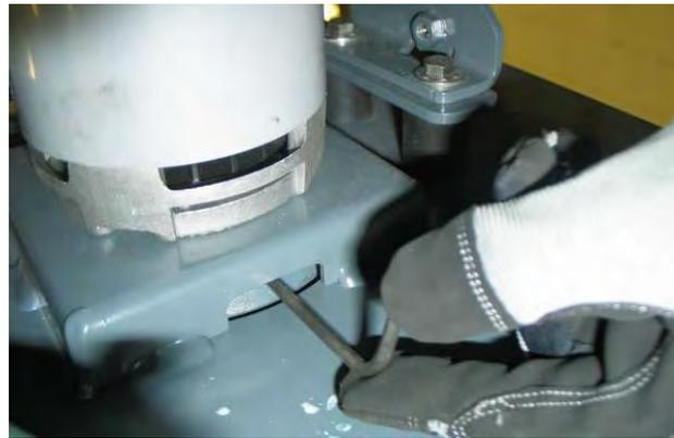
6. Remove the lower plate and the lower isolators (4).
