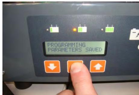
5. Press the middle button to select the battery type. The red LED light will turn off.
