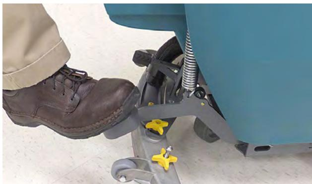
9. Loosen (do not remove) the RH side linkage bolt.
