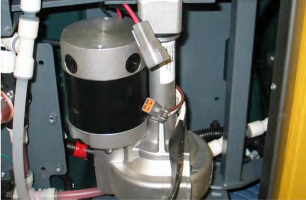
3. Turn off ec-H<sub>2</sub>O (if equipped) and disconnect the conventional water valve from the wire harness.
