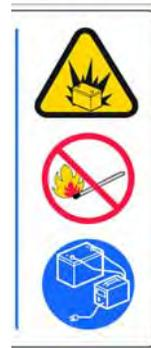
**WARNING LABEL - Batteries emit hydrogen gas. Explosion or fire can result. Keep sparks and open flame away when charging.**
