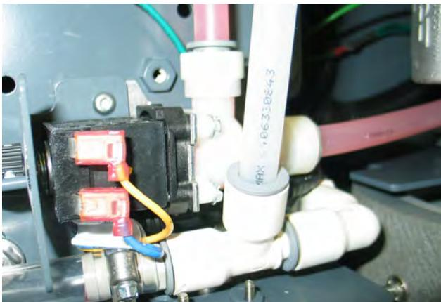
3. Disconnect transaxle motor (option) electrical connector.
