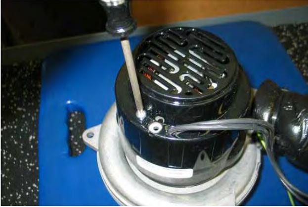
2. Loosen carbon brush mounting torx screws (4).
