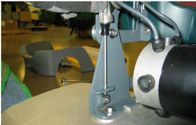
11. Re-apply chalk and repeat steps 4-10 until the desired brush pattern is achieved and then retighten the linkage bolt with the **HEAD IN THE LOWERED POSITION**.
