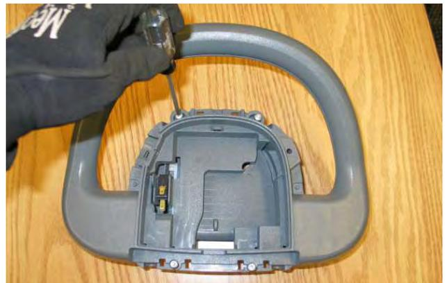
13. Remove screws (9) from rear of operator's console and separate console assembly.
