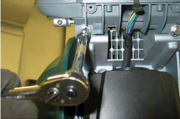
9. Lift up and forward to remove the operator console and place console on a work bench.
