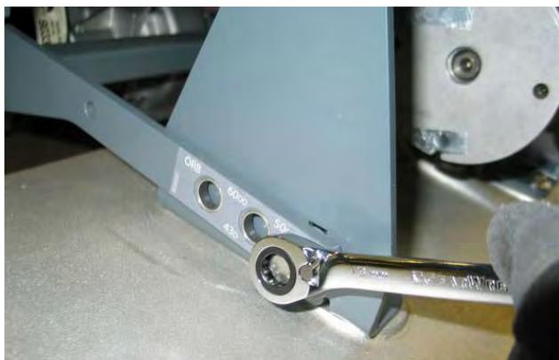
10. Turn the adjustment screw counter-clockwise to increase down pressure on the RH side or clockwise to decrease down pressure on the RH side of the scrub brushes.
