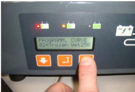
7. Press the middle button to save the new settings. The screen will display "PROGRAMMING PARAMETERS SAVED".
