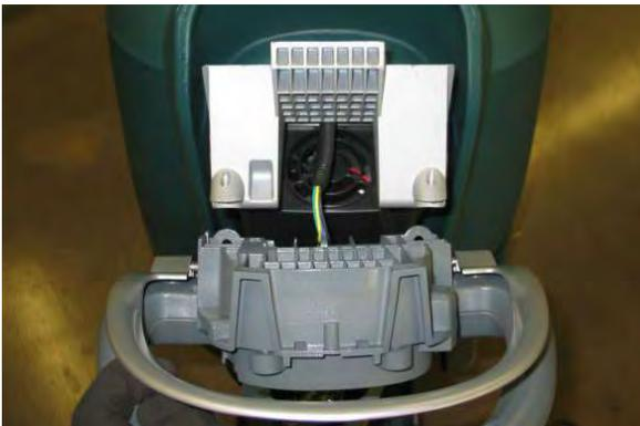
10. Remove plastic knobs and set aside. If replacing the potentiometer or directional switch, use a socket to remove the nut securing the potentiometer or the directional switch.
