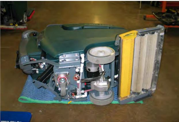
6. Remove wheel nuts (2). It will be necessary to raise the machine up and lower it to the right side to access the left side wheel.
