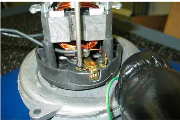
3. Lift up to release and remove carbon brushes (2).
