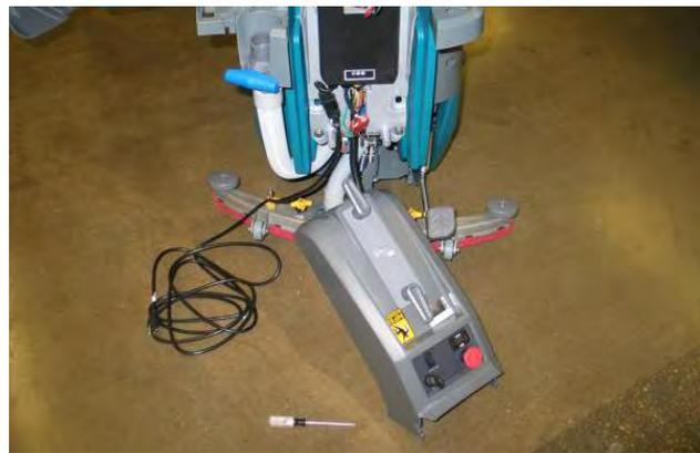
4. Remove four (4) hex screws to remove the control console plate.
