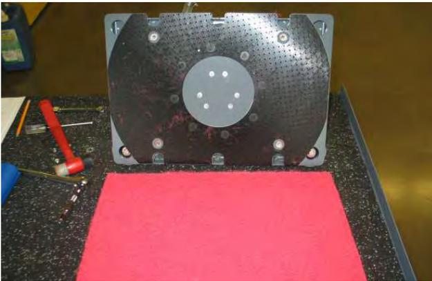
4. Remove flat head screws securing the lower plate to the lower isolators.
