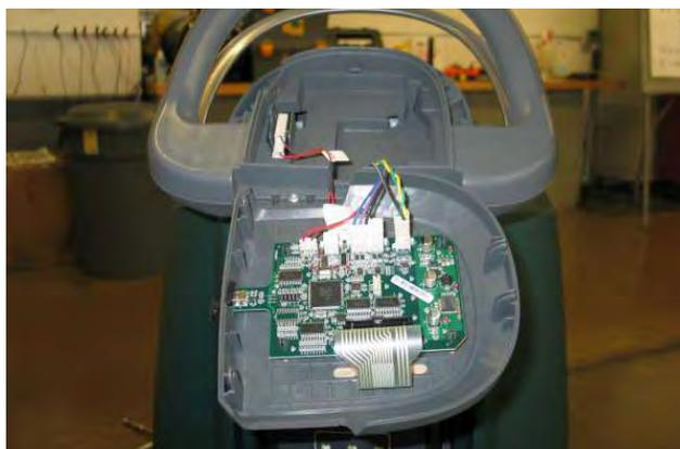
7. Disconnect electrical connections and remove interface module.
