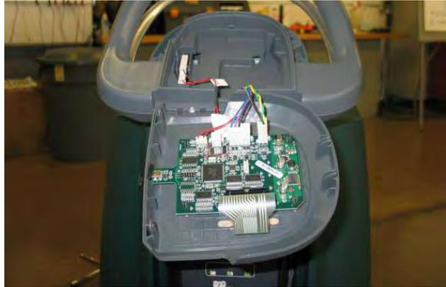
6. Remove T-25 torx mounting screw (1).
