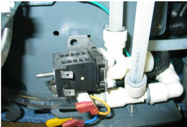
8. Disconnect PTC (Push-To-Connect) connections (2) from solenoid. See *PTC (PUSH-TO-CONNECT) FITTINGS* in the *SERVICE* section of this manual.
