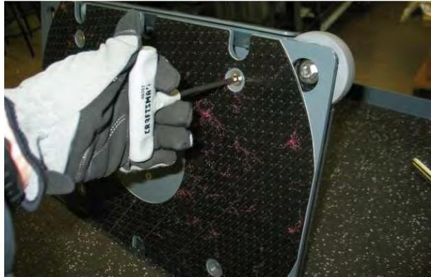
5. Loosen the 4 mm set screw securing the concentric motor weight to the motor shaft.
