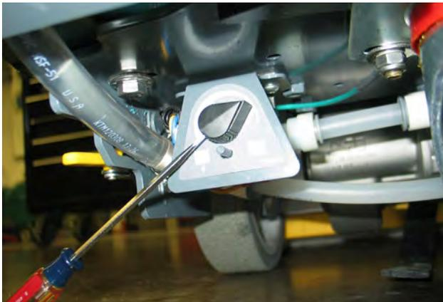
2. Disconnect scrub head side PTC (Push-To-Connect) fitting from water solenoid. See *PTC (PUSH-TO-CONNECT) FITTINGS* in the *SERVICE* section of this manual.
