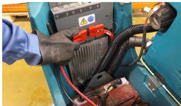
3. Remove batteries and set aside.
