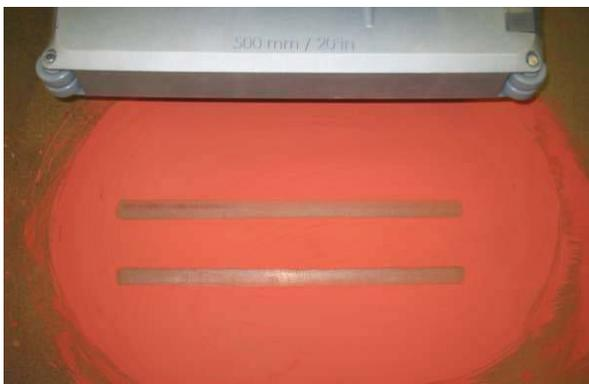
12. The taper adjustment is complete. If the pattern is uneven front-to-rear, the brush pattern can be further adjusted using the slotted top bolt. Loosen the top bolt just enough so the scrub head bracket moves freely and the scrub head settles in it's natural position on the level floor.
