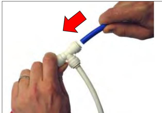
3. Push into the tube stop. The collet has stainless steel teeth which hold the tube firmly in position while the o-ring provides a permanent leak-proof seal.
