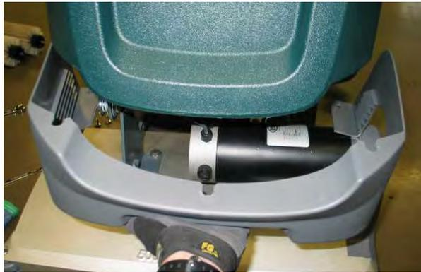
7. Disconnect motor from wire harness connection.
