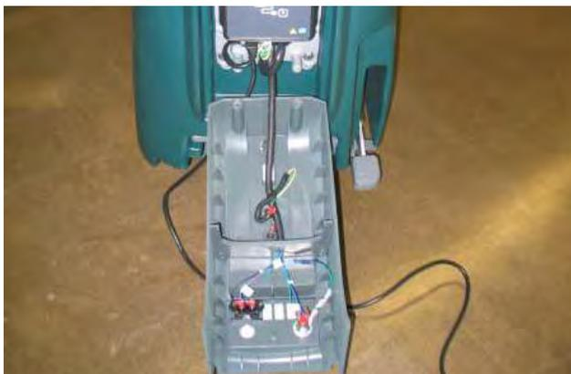
5. Remove T-25 torx mounting screws (2).
