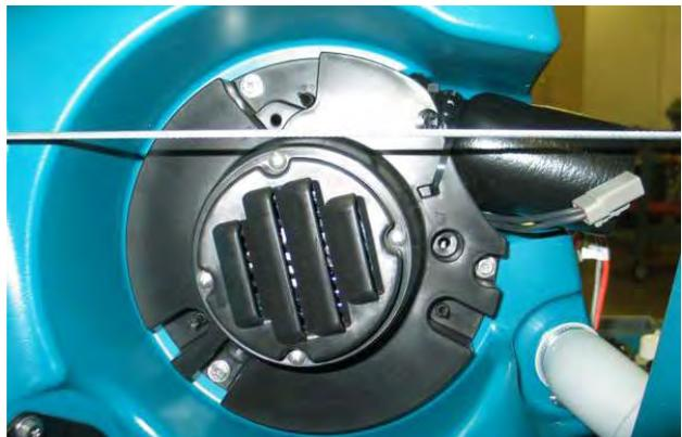
4. Remove vacuum fan mounting hardware (3).
