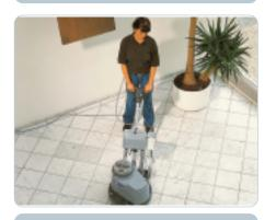
This high-speed unit features 3-step integrated active dust extraction for dust-free, polymer film coat renovation. This means that hard floors can be cleaned and polished without the inconvenience of conventional water and chemical usage. Fantastic productivity gains can be achieved.
