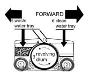
Two counter-rotating brushes (1 and 2) throw the soiled water on to the revolving drum (3), from there it is fed into the waste water tray (5) by means of a stripper blade (4).
