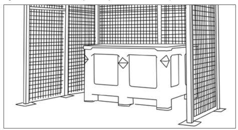
An example of a well protected area with a cage to protect against accidental impact damage and with the batteries stored in a protective container to protect from heat, impact and accidental spillage of liquids.
