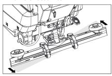
→ Tighten the wing screws.
