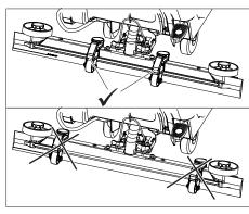
→ Check if the height adjustment is mounted on the inside of the vacuum bar.
