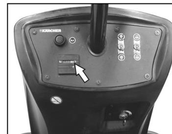
Elapsed-time meter indicates maintenance interval times.
