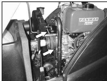
Check round belts and V-belts for tightness, wear and damage
