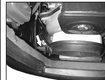
Freewheel lever of axle drive must be in its bottom position
