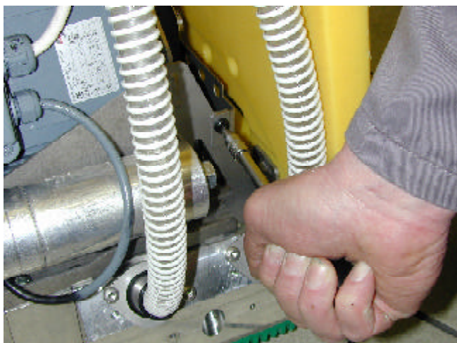
Remove the retaining bolt and protection cover
