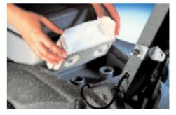
Burnishing can raise dust. The dust extraction solves the problem with a disposable filter and easily changed collector bag.
